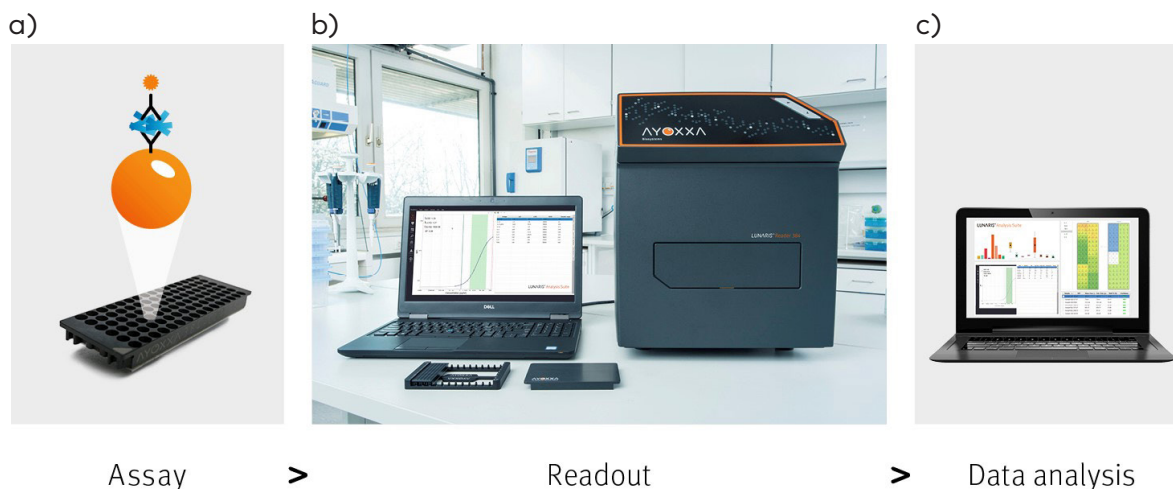
Figure 2: Schematic of the LUNARIS multiplex procedure. (A) The LUNARIS assay follows the classical sandwich ELISA principle. Samples are added to each well of the BioChip and targeted analytes are captured by the antibody-coated beads during incubation. The wells are washed and the captured analytes are labelled with biotinylated detection antibodies and streptavidin-phycoerythrin (SA-PE). The plates are air dried and subsequently imaged with the LUNARIS Reader (B) to quantify the fluorescence signal on the beads. (C) The LUNARIS Analysis Suite Software provides a tailored report with detailed information on the concentration of targeted proteins in each sample.
